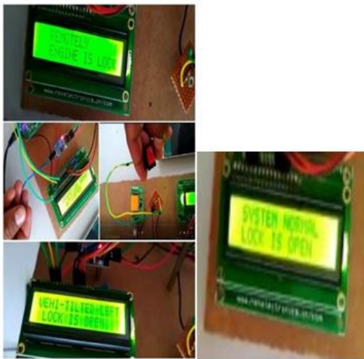
Figure 4. LCD read when functions are activated: (a) LCD displaying when engine is locked, vehicle fall is detected, ignition lock and vibration sensor is activated. (b) LCD read when system is normal.
