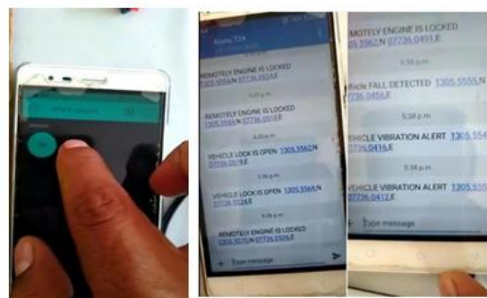
Figure 3. Application of the app: (a) locking engine through app. (b) messages received when engine is locked, vibration sensor is activated & vehicle fall is detected with GPS position.
